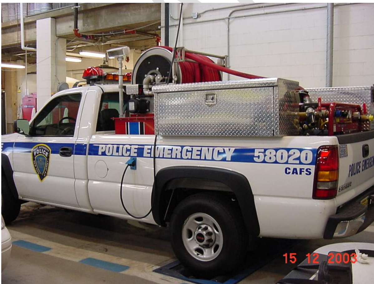
Figure 5. QRV Deployed as Front-line Fire Suppression Vehicle
